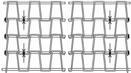
All welded selvage belts over 24 inches in width feature the resistance welding of every other connector rod to the flat strip on the 2nd opening in from each edge of the belt. On True 1/2" x 1/2" mesh belts this weld is on every 3rd connector rod.
